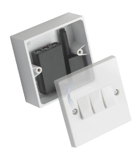
Using the easyswitch EST-1 transmitter module allows you to adapt any make or style of plate switch in to a radio transmitter switch for controlling remote lighting. The switch can be surface or flush mounted and may be Single, Double, Triple or Quad gang to operate up to four zones.
